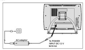
IMPORTANT: The TV set is designed to operate on 12 V DC. For this, an adaptor is used which gives 12V DC voltage. Connect this adaptor to a system that supplies 220-240V AC, 50 Hz.
