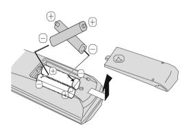
**NOTE:** Remove the batteries from remote control handset when it is not to be used for a long period. Otherwise it can be damaged due to any leakage of battery.
